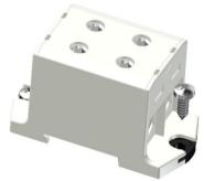
**Screw mounting** Use max. Ø5 mm screw. See picture.
