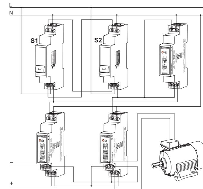
The motor control system with rotation direction changing.
