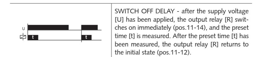
SWITCH OFF DELAY - after the supply voltage [U] has been applied, the output relay [R] switches on immediately (pos.11-14), and the preset time [t] is measured. After the preset time [t] has been measured, the output relay [R] returns to the initial state (pos.11-12).
