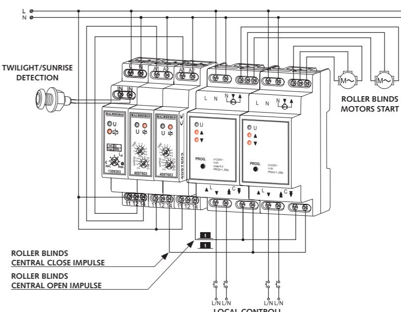
4097603 time relay cooperates with the 1309303 twilight switch and with roller blinds controller. Its function is impulse generation at dusk. This impulse is a signal for the roller blinds controllers (central closing input) and for moving down all the roller blinds working in the same group.
