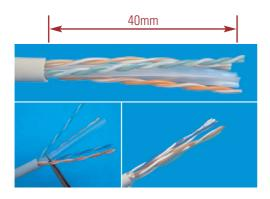
2. Follow the color-coding to position T568A or T568B wiring.
